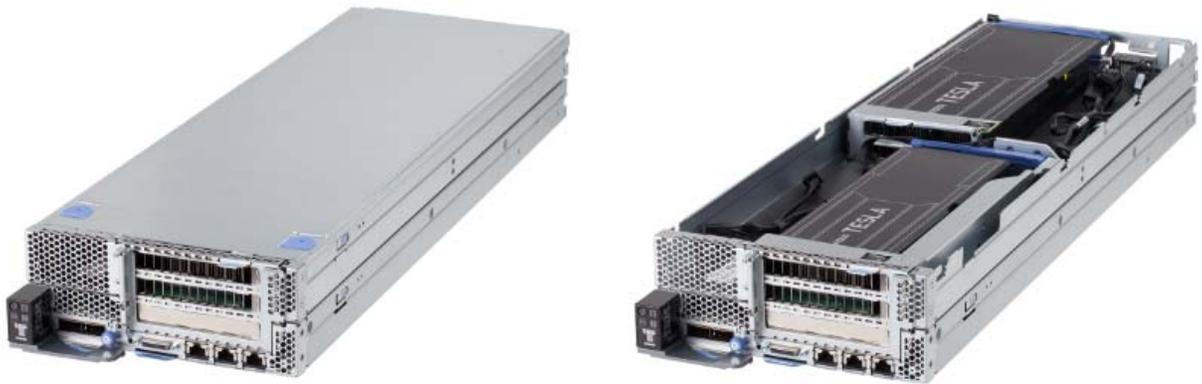
Figure 5: NeXtScale nx360 showing GPU tray with two double height GPUs
