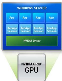
Figure 9: Citrix XenApp Sharing of a GPU
