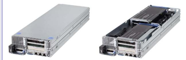
*Figure 5: NeXtScale nx360 showing GPU tray with two double height GPUs* The six compute nodes are installed in the IBM NeXtScale n1200 enclosure as shown in Figure 6.
